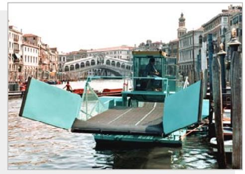
Our existing harvester design was easily evolved into a vessel that could pick up floating debris, and thus the trash skimmer was born.
