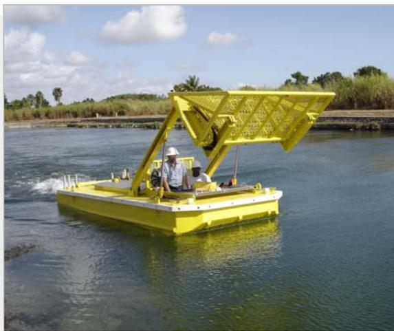
The Weed Tow Boats are designed to clean nuisance aquatic plants out of deep water drainage canals. Outfitted with a plow that is lowered off the stern and dragged along the channel bottom, vegetation is ripped loose at the roots. The severed weeds then float to the surface and are scooped up in the front end loader to be deposited on shore for disposal.
